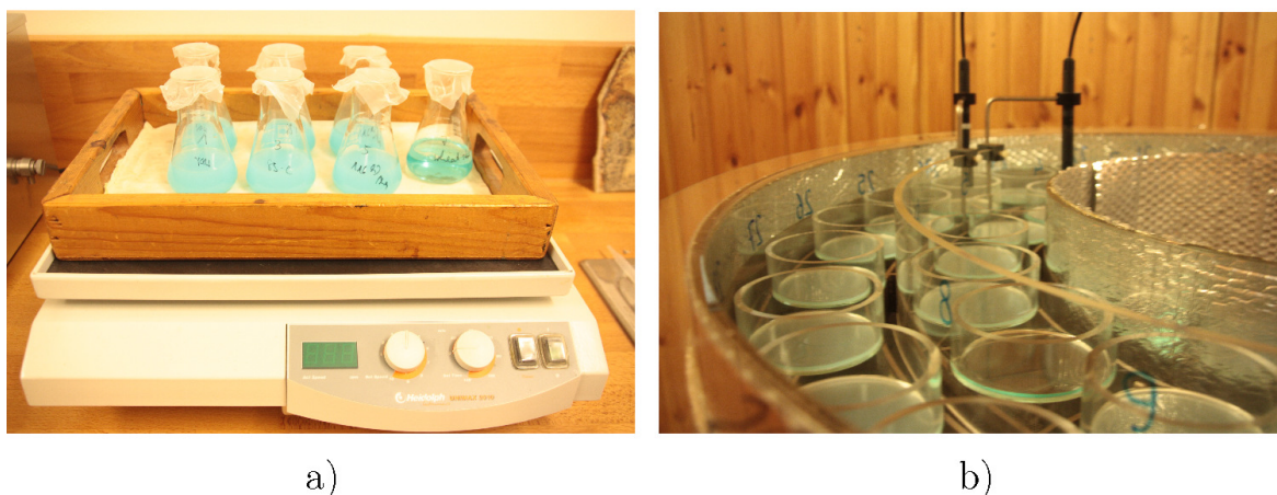
Figure 3.10: a) preparation of the mixtures for the biocrystallization experiment: final stirring, b) pipetted samples in dishes inside the inner chamber with two sensors for temperature and humidity monitoring. Cloudy mixtures: milk samples, clear-transparent samples: wheat standard.
