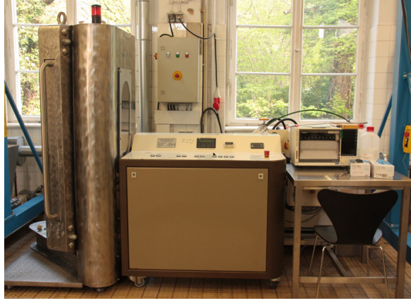
Figure 3.2: HP-unit single Vessel U4000, closed.
