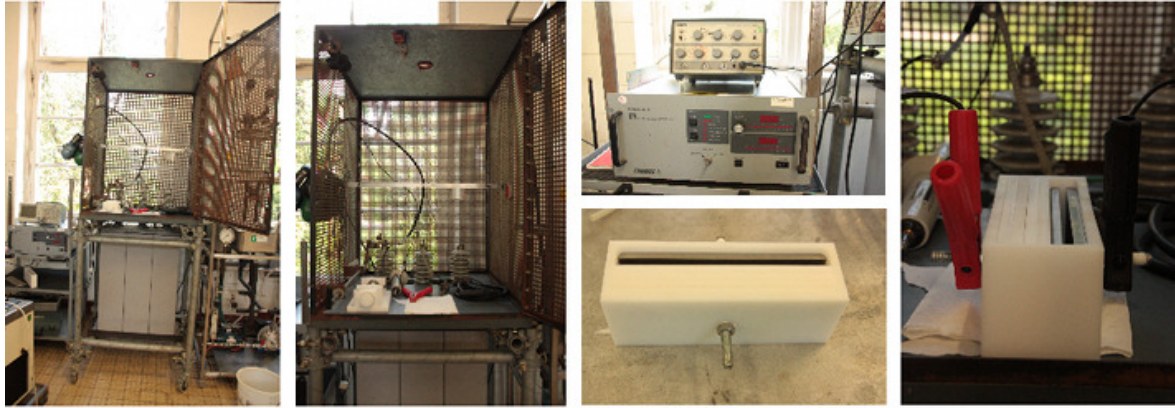
Figure 3.3: PEF-unit: a) view on the entire unit, b) treatment chamber, c) (above image) frequency generator (top) and power supply (below image), d) (bottom) parallel plate treatment chamber and e) connected parallel plate treatment chamber (without sample).
